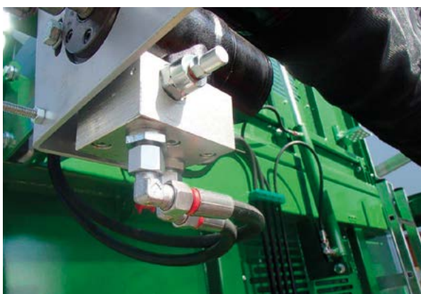
Safety element: Pressure control valve
