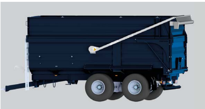
Flexcover Fix – winding from the rear of the trailer
